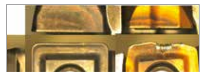
Competitor B 140 Holes (13 m) Wear and chipping on cutting edge
