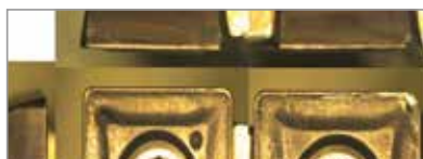
Competitor A 230 Holes (21 m) Chipping on cutting edge
