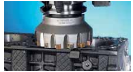
Roughing for cast iron
